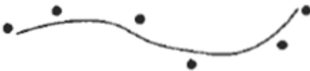
Figure 10-20 A set of six control points approximated with piecewise continuous polynomial sections
