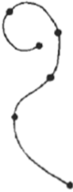
Figure 10-19 A set of six control points interpolated with piecewise continuous polynomial sections.
